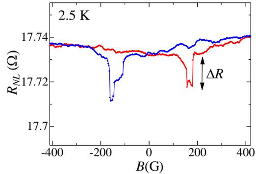
Fig. 2: Nonlocal MR in organic NLSV. Nonlocal resistance decreased at the antiparallel configuration of FM electrodes.
