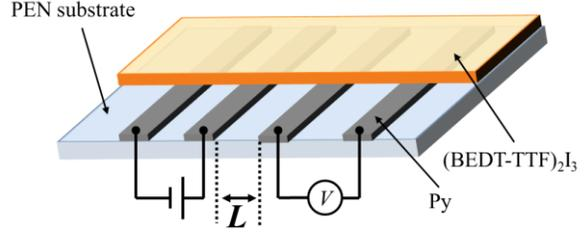
Fig. 1: Schematic of NLSV.
