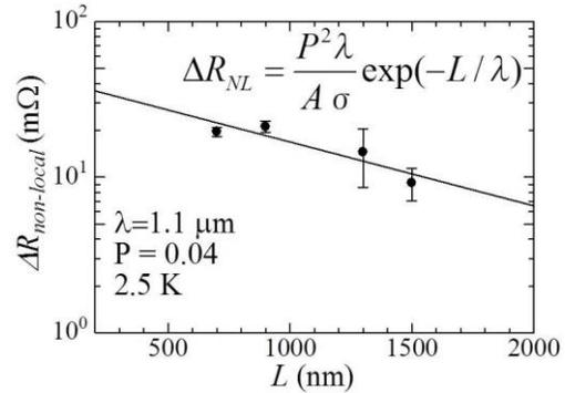
Fig. 3: Plot of non-local MR as a function of the spacing between electrodes.
