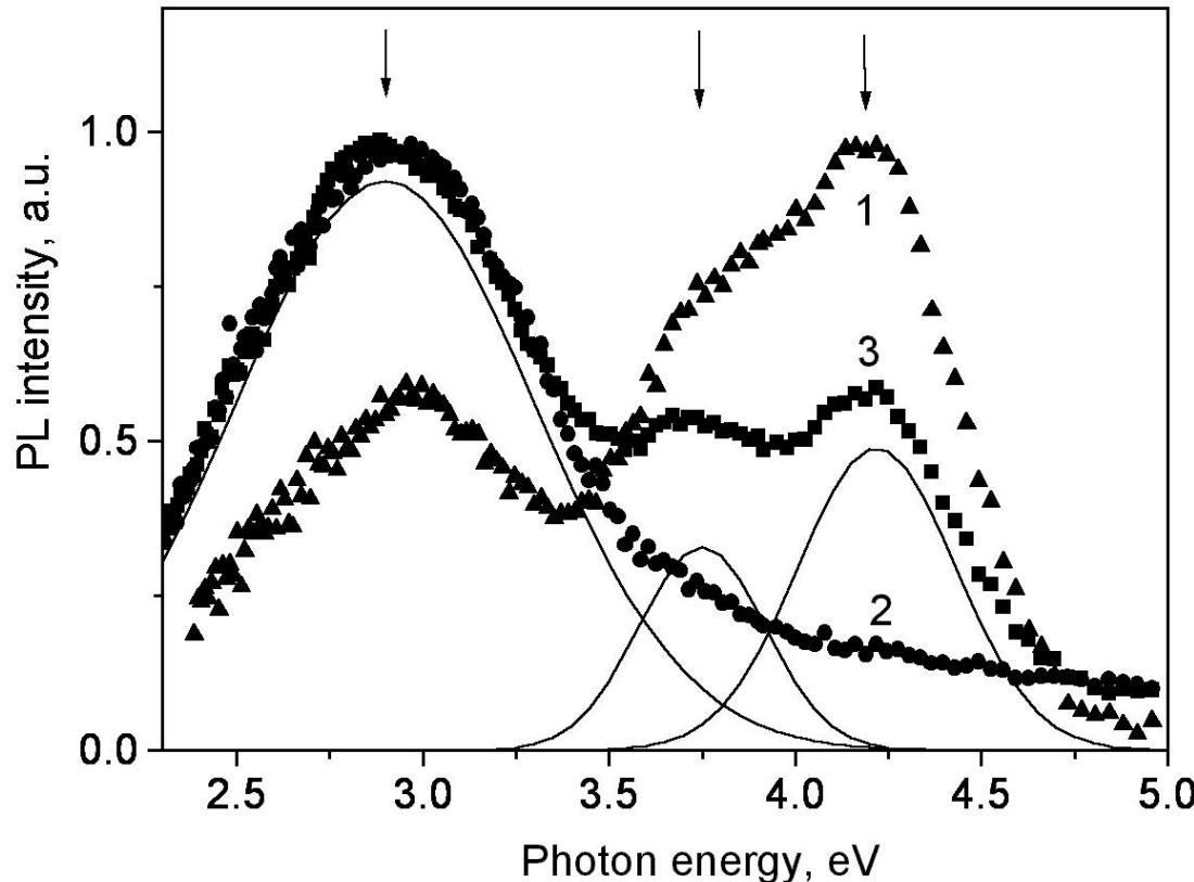
Photoluminescence energy indicate on existence of oxygen vacancies in  $\text{Al}_2\text{O}_3$
