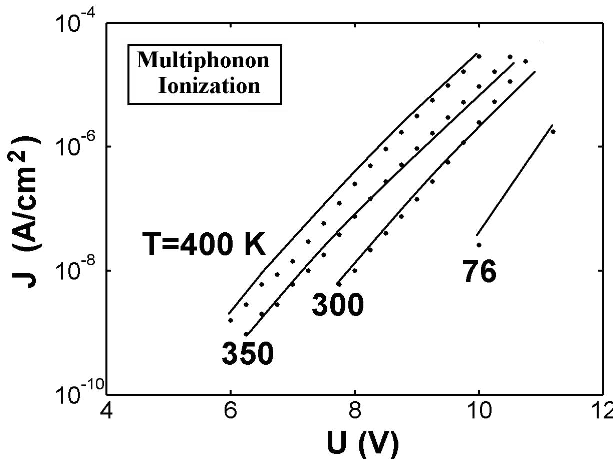
Thermal trap energy  $W_t = 1.5 \text{ eV}$  (half of Stokes shift)
