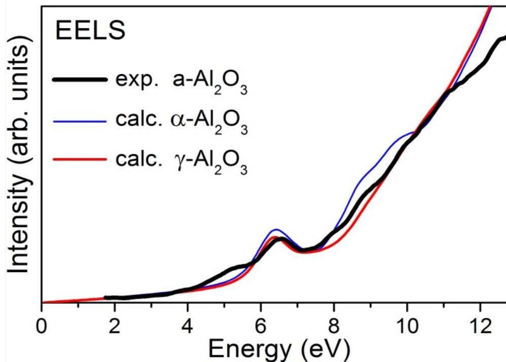
Experimental EELS spectra for a- $\text{Al}_2\text{O}_3$  (black line) and calculated one for  $\alpha$ - and  $\gamma$ - $\text{Al}_2\text{O}_3$  with oxygen vacancy.
