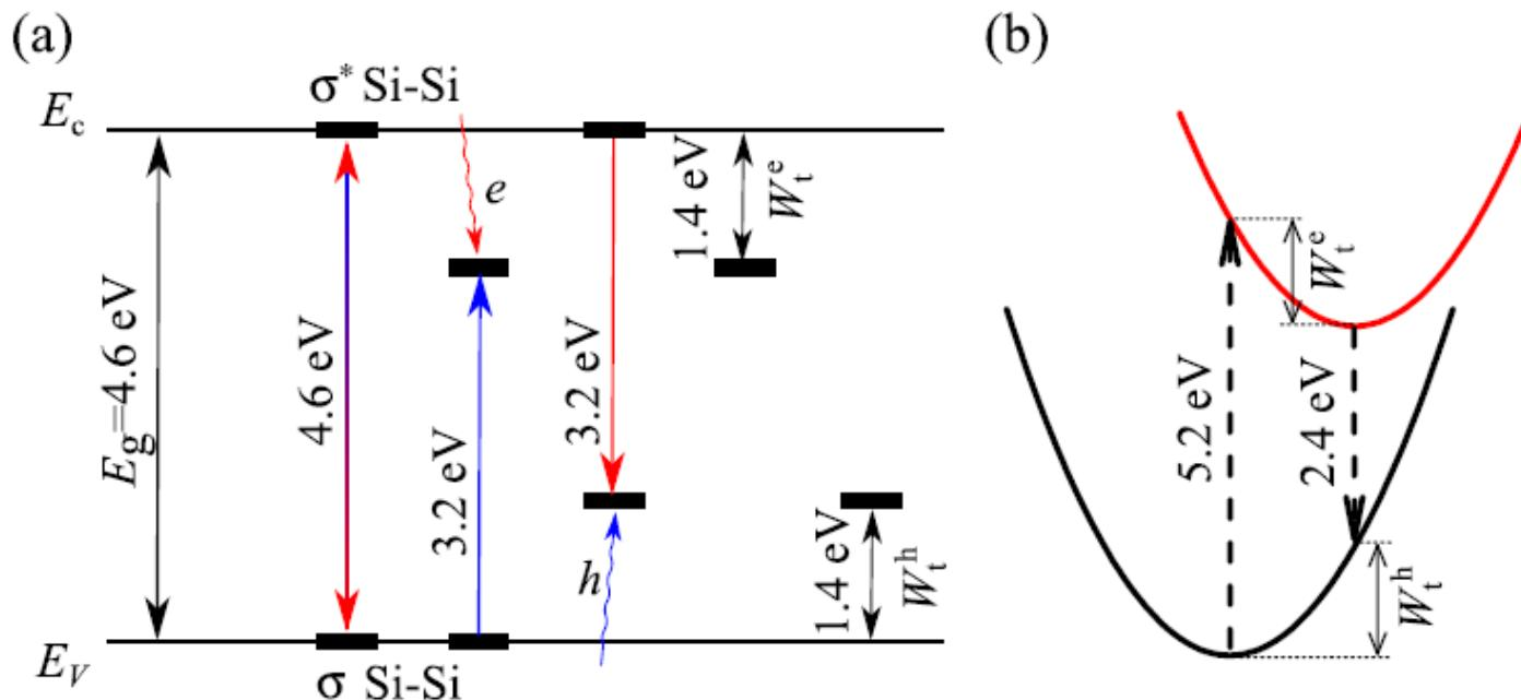
FIG. 5. (a) The energy diagram of electronic transitions in the Si–Si bond in  $\text{Si}_3\text{N}_4$  associated with the UV PL. (b) A configuration diagram of the optical transitions related to the 2.4 eV green photoluminescence line in  $\text{Si}_3\text{N}_4$ .
