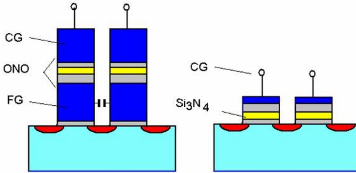
The substantial disadvantage of floating gate flash memory is parasitic interference during information writing. Interference results in low reliability of flash memory and restriction for scaling to increase memory volume  $> 64\text{Gbite}$ . This disadvantage is overcome in charge trap memory based on  $\text{Si}_3\text{N}_4$ .
