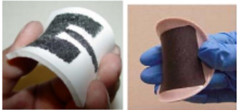
Fig. 1 Very flexible E-textile antenna printed on polymer
