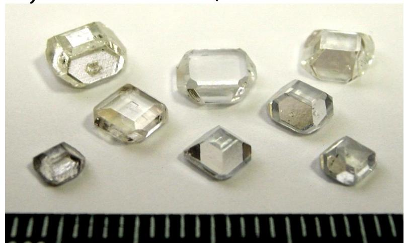
{100} IIa type crystal with the area up to 30 mm<sup>2</sup> was grown using (111) seed orientation for 2-3 carat size
