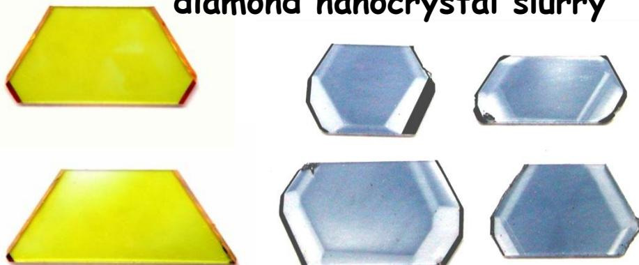
200-400 µm plates of {111} plates with the area up to 25 mm<sup>2</sup> were produced by laser pointing with subsequent cleavage along the plane of the spikes, grinding & polishing or CVD overgrowth.
