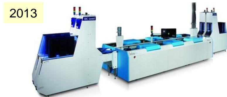
Production tool for 10 nm  $\text{Al}_2\text{O}_3$
