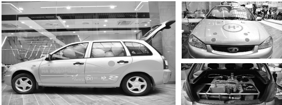
The first Russian electric car with ASTRA fuel cell range extender. It increased its range from 200 km to 400 km.
